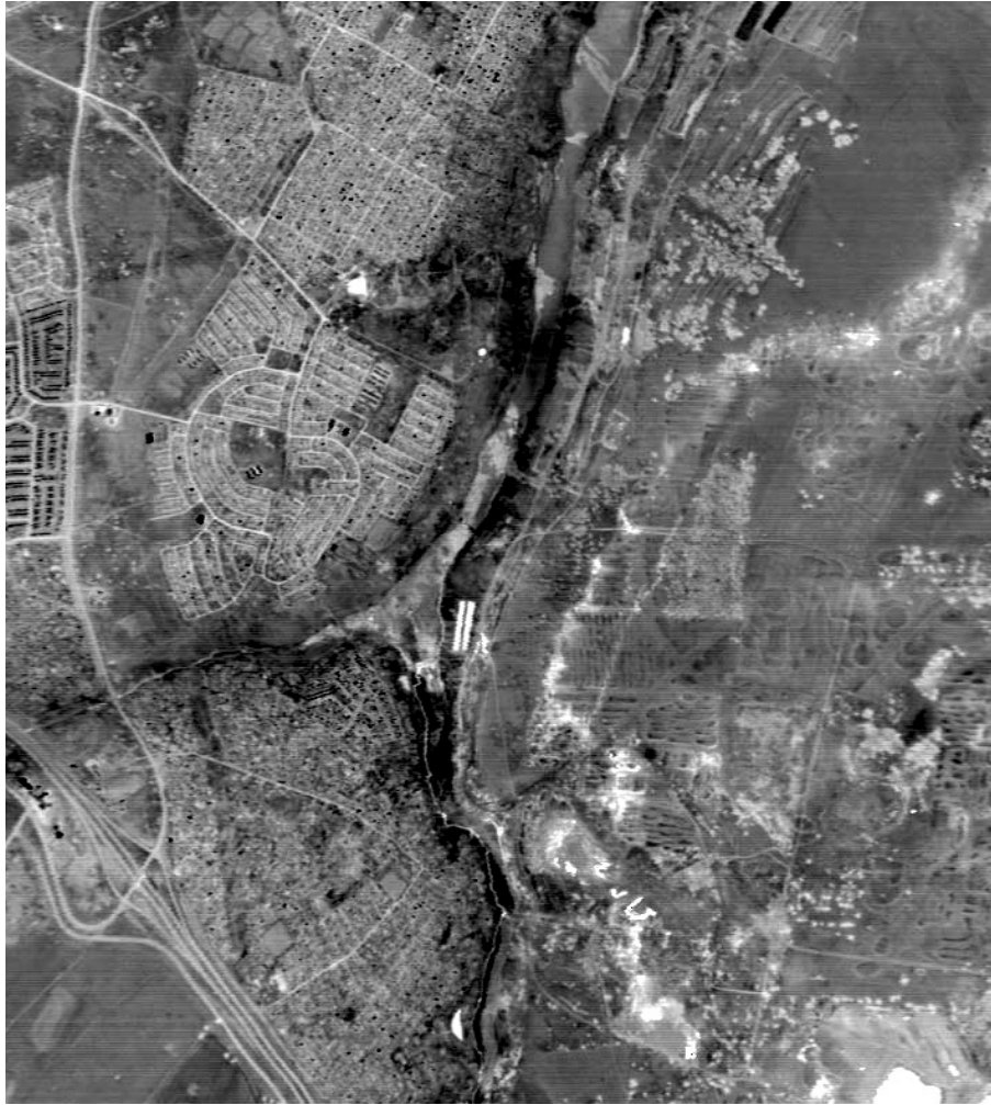
Figure 5: Airborne LWTIR image with 5 metre resolution, over the old T & DB Colliery west of Witbank taken in pre-dawn conditions in 1998.
