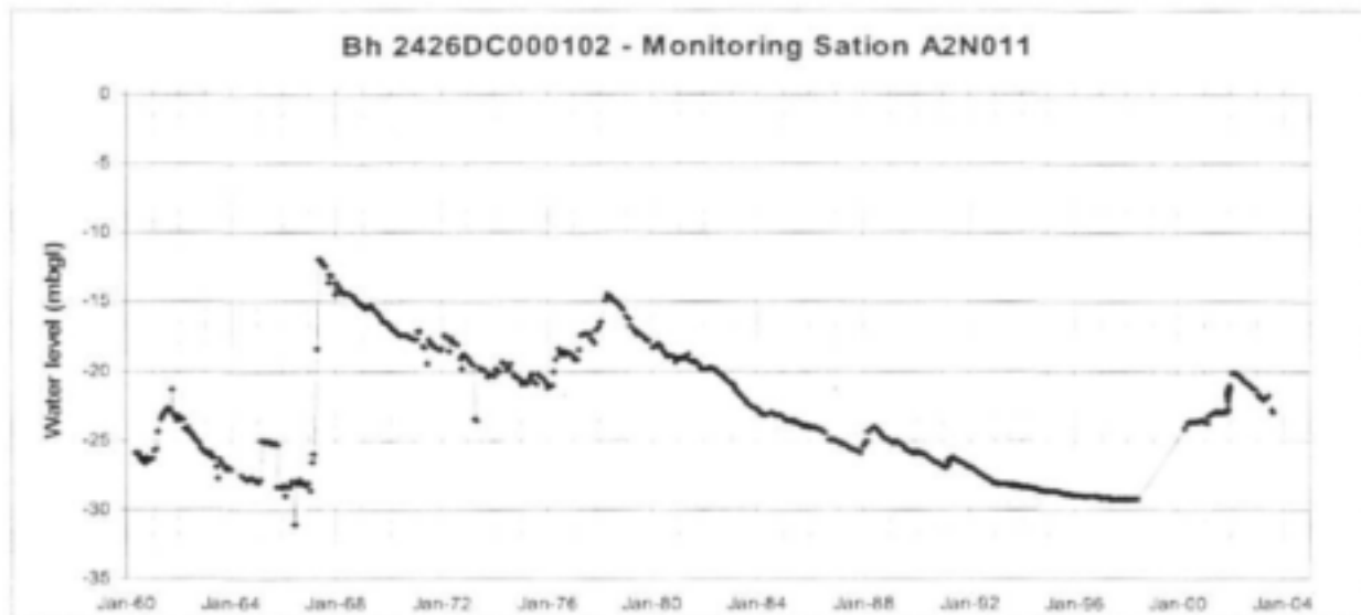
Figure 8: Water level graph for borehole 2426DC000102, Groundwater level monitoring station A2N011, some 30km north of Pilanesberg on the farm Parys.
