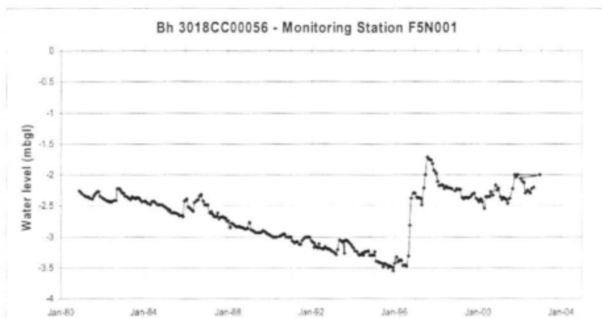
Figure 10: Water level graph for borehole 3018CC00056, groundwater level monitoring station F5N001, approximately 100km northwest of Van Rhynsdorp on the farm Moordenaarskraal.
