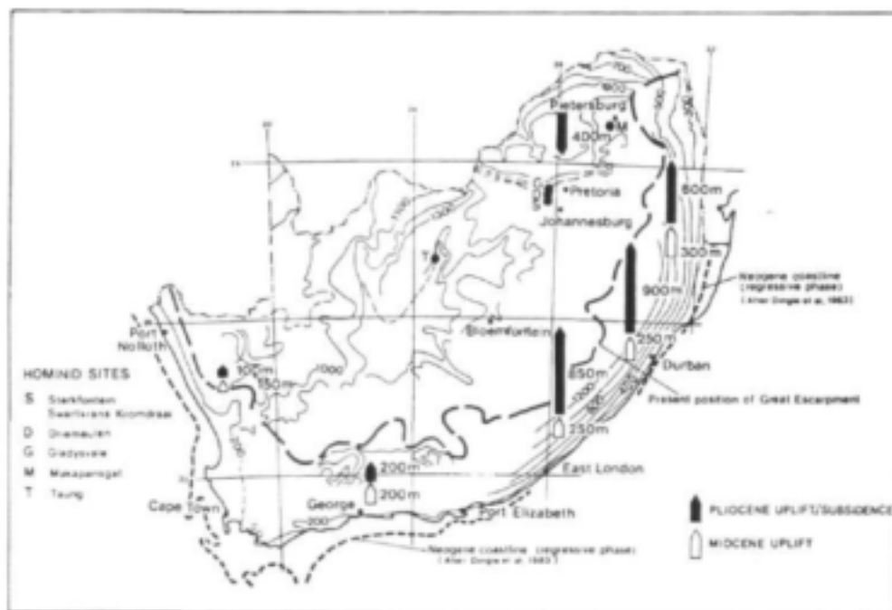
Figure A-5: General contours on the Post-African Miocene erosion surface. Open arrows indicate the uplift during the early Miocene, while solid arrows show the uplift or subsidence during the Pliocene (Partridge, 1997).
