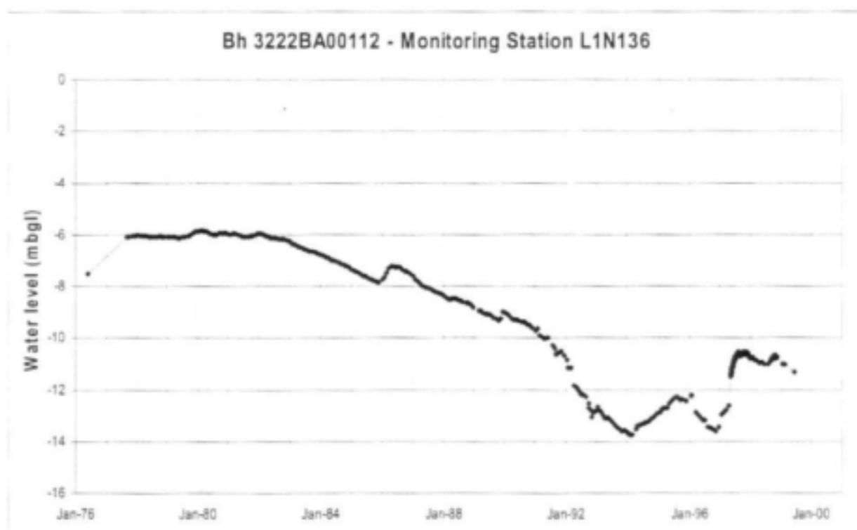
Figure 11: Water level graph for borehole 3222BA00112, groundwater level monitoring station L1N136 approximately 80 km northeast of Beaufort West on the farm De Hoop.
