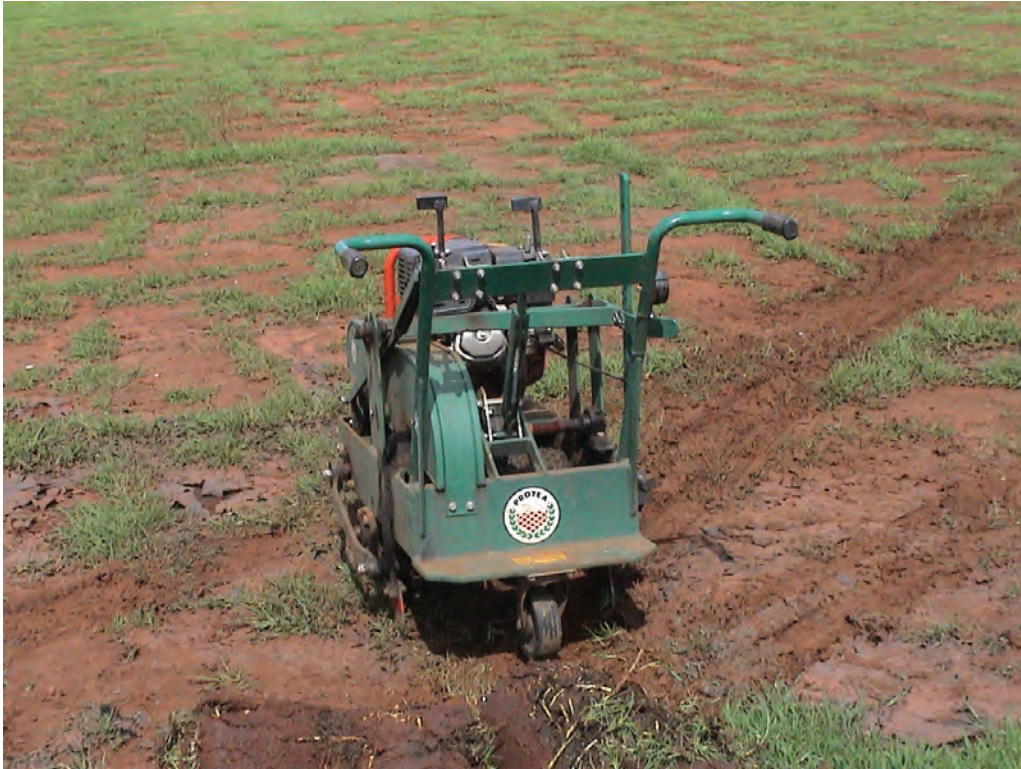
Figure 7.4 A hand operated, light-weight, petrol powered sod cutter
