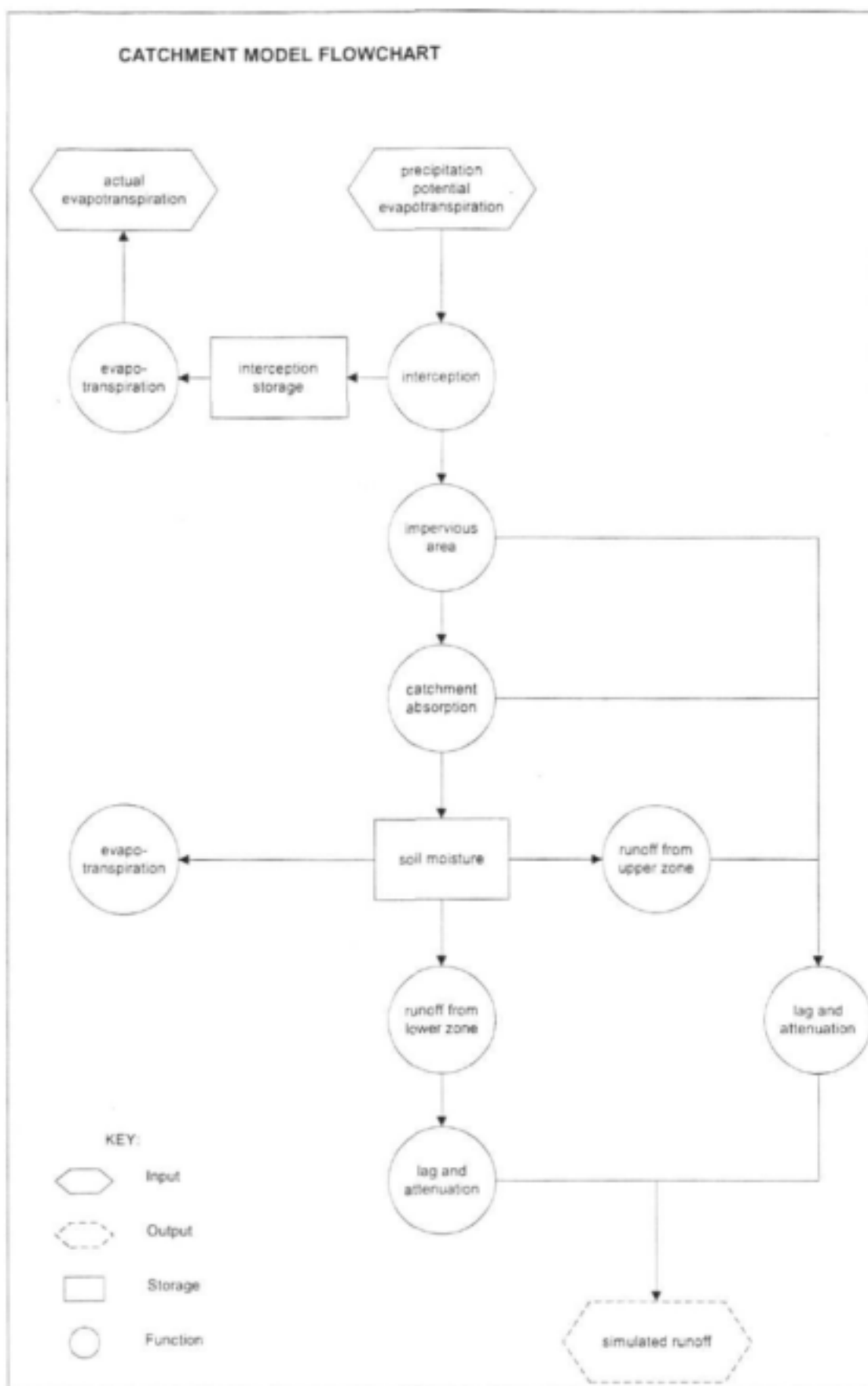
Figure 3-1: Pitman Catchment Model Flow Chart (HRU, 1973)
