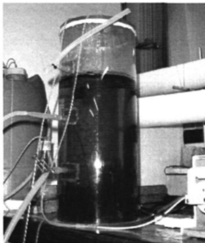
Figure 4.9: The selective precipitation vessel showing the formation of the brown copper and lead sulphide precipitate.
