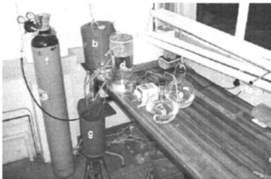
Figure 4.8: Bench scale integrated biological system showing the various components, a = anaerobic digester feed, b = 28l anaerobic digester, c = algal gutters, d = selective precipitation vessel, e = acid mine drainage, f = nitrogen source and g = precipitation vessel.
