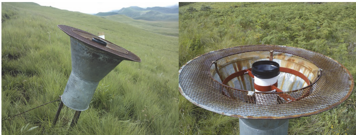
Figure 3.18: A Snowdon raingauge with Nipher shield at the angle of the slope, with a vertically positioned Texas raingauge in the background (left). Replica of the historically used Snowdon raingauge placed within the Nipher shield (right)
