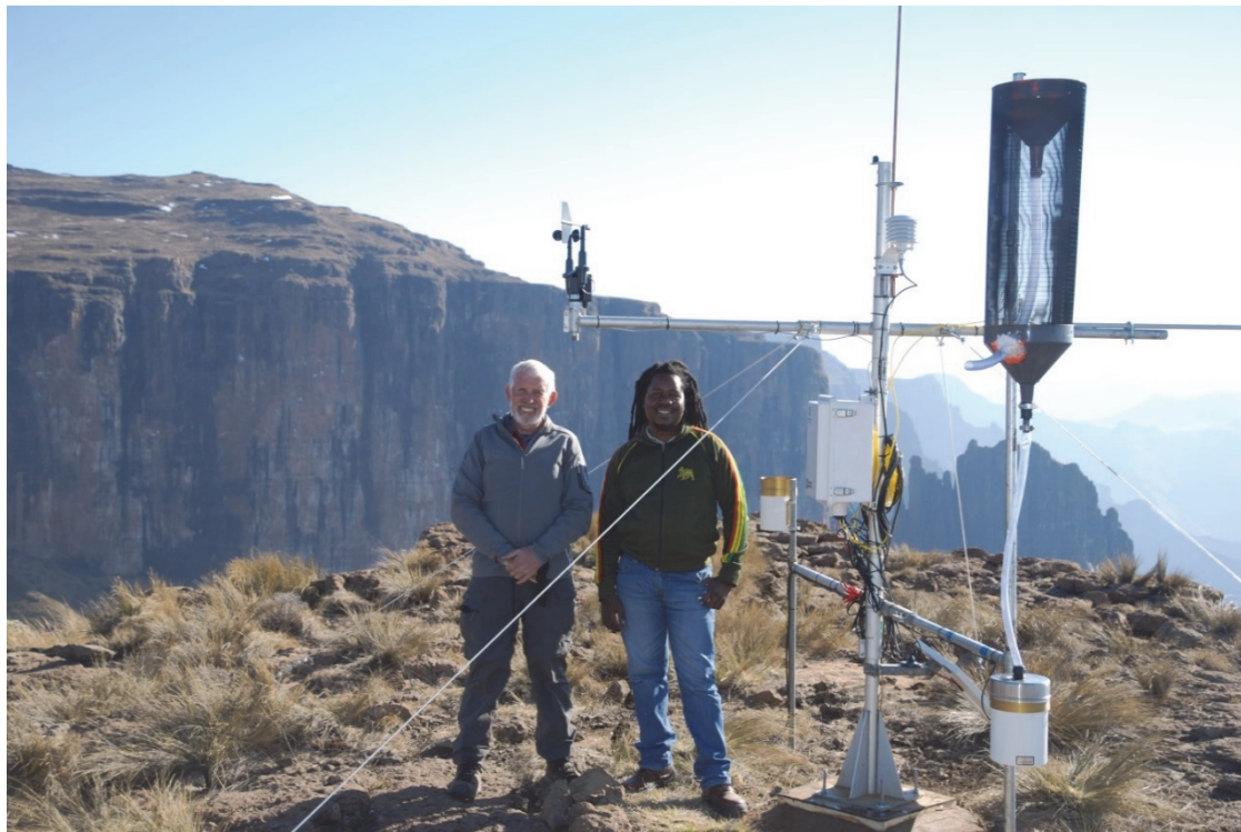
Figure 3.10: Campbell Scientific automatic weather station on the Drakensberg escarpment. A normal raingauge (in the background) and a fog-gauge (foreground) have been installed to monitor precipitation
