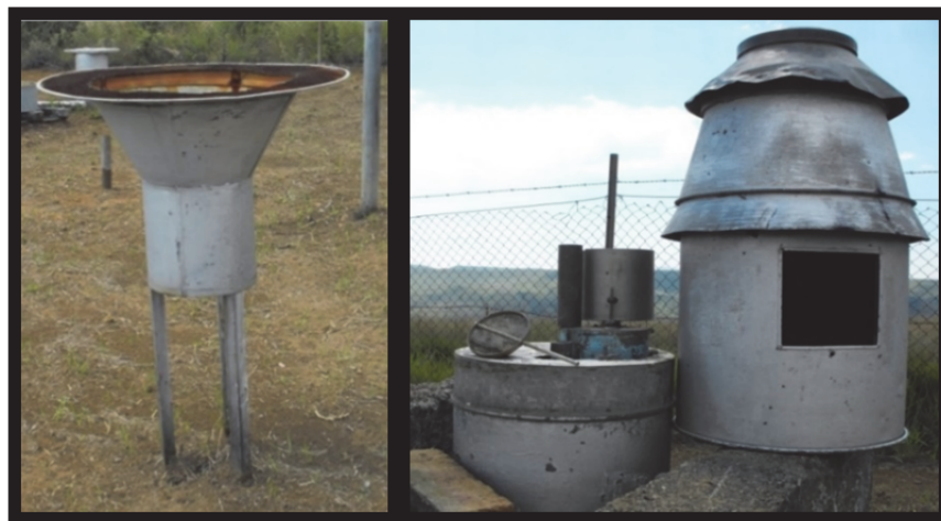
Figure 3.2: Historical raingauge types used in the Cathedral Peak research catchments, left 5" Snowdon gauge equipped with Nipher shield, right Casella Snowden 5 & 1/16" recording raingauge
