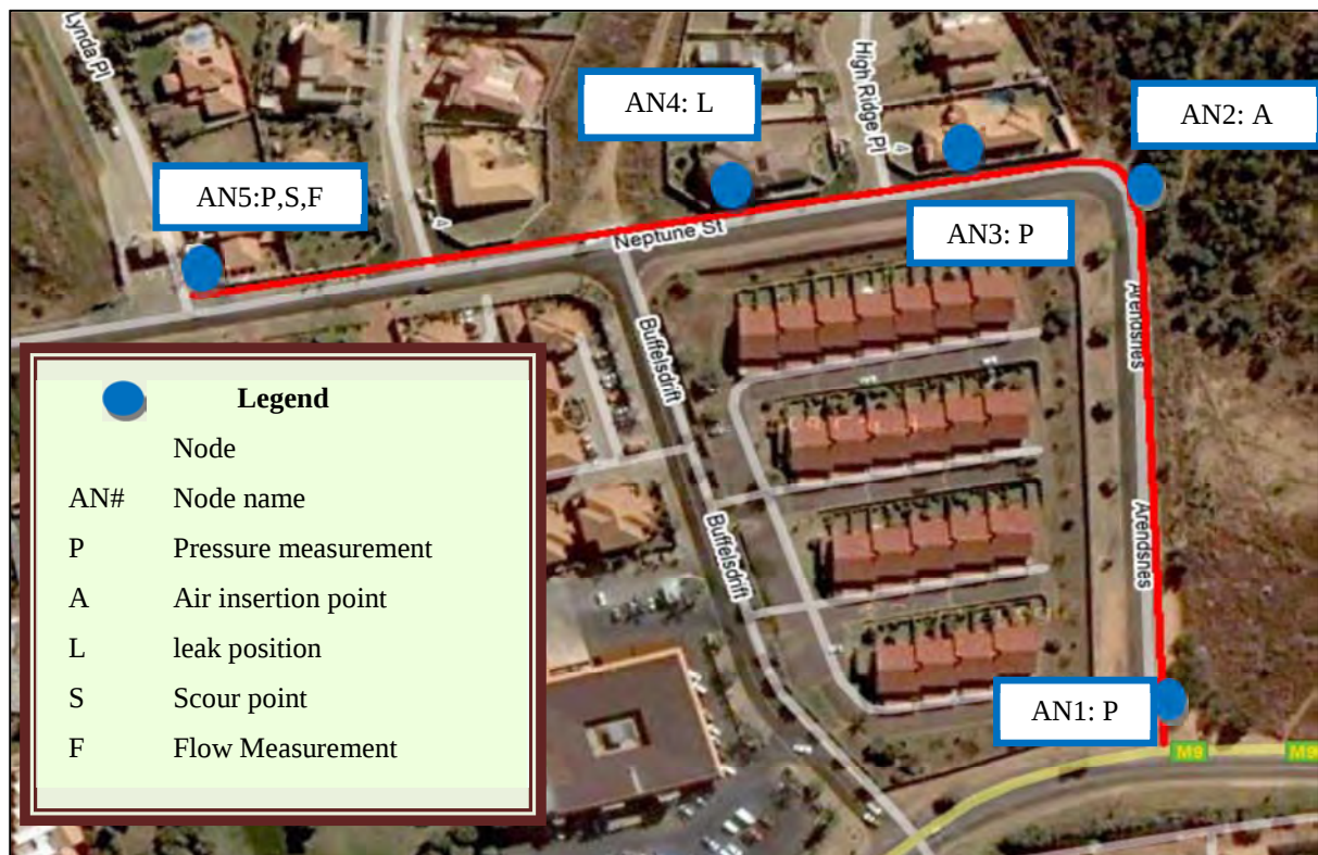
Figure 4-2: Positions where instrumentation was installed on the Arendsnes pipeline
