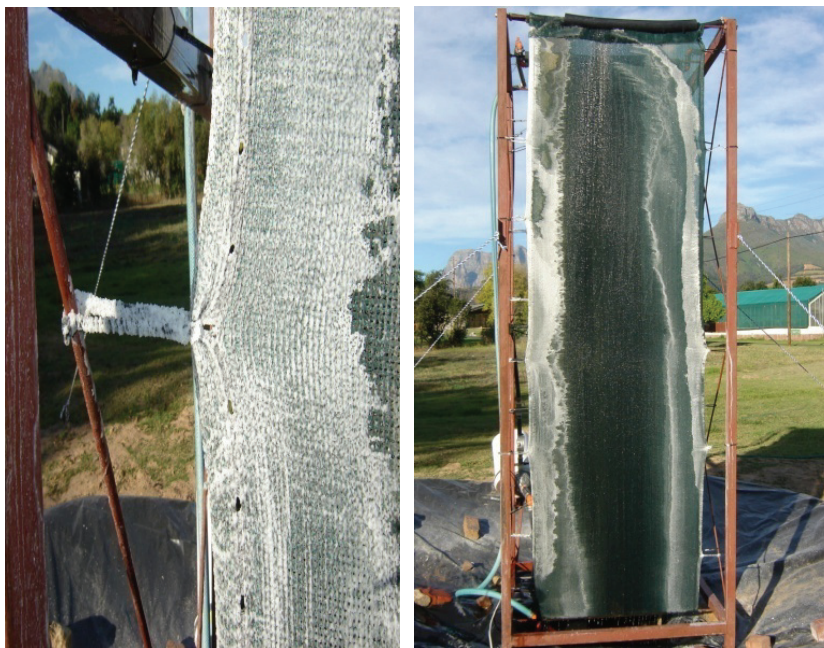
FIGURE 73. WHITE SODIUM CHLORIDE CRYSTALS ON WAIV NETTING
