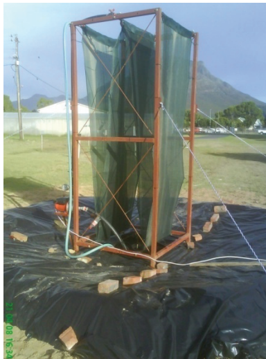
FIGURE 70. LINED AREA AROUND WAIV UNIT.
