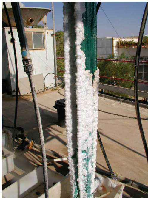
FIGURE 31. CRYSTAL FORMATION ON WAIV SURFACES
