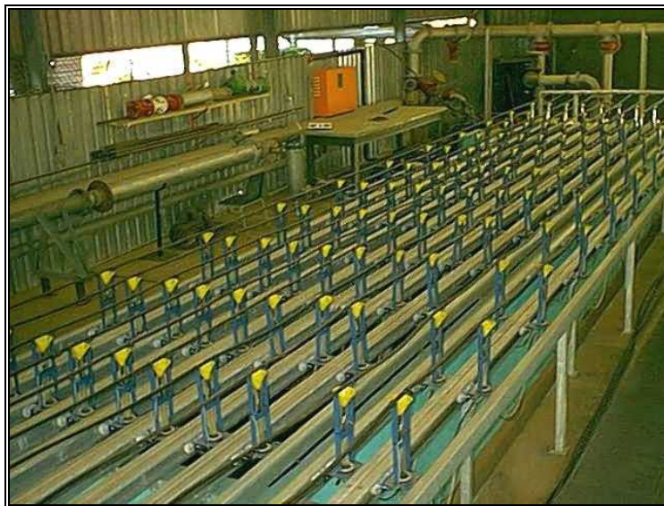
Fig. 2: Test bench for emitter discharge and CV_q tests
