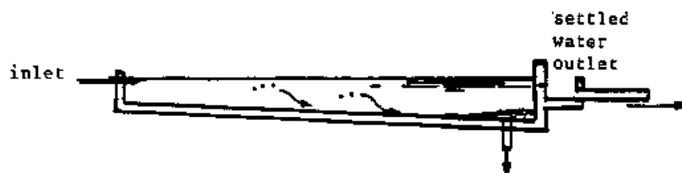
Fig. 2.5 Horizontal flow sedimentation tank
