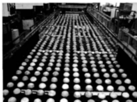
Figure C-17 Pattern H1 spacing cross-sectional 0.110m, longitudinal 0.167m
