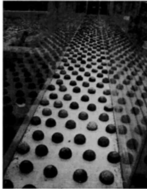
Figure 3-1 Arrangement of roughness elements in Flume B (Test 1.1.5 shown)
