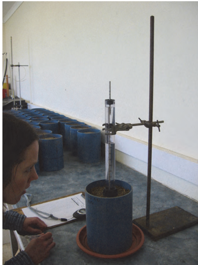
Figure 10.3. Using a mini disk infiltrometer to measure K in the laboratory at the ARC Nietvoorbij campus.
