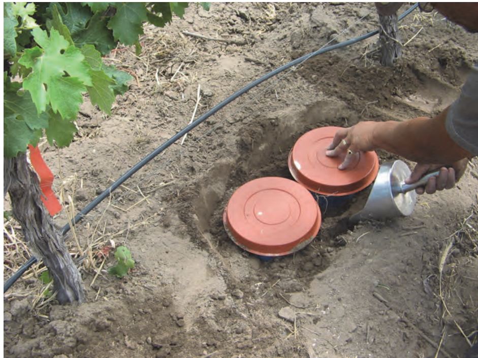
Figure 10.2. Soil from the vineyard was used to fill up the hole.
