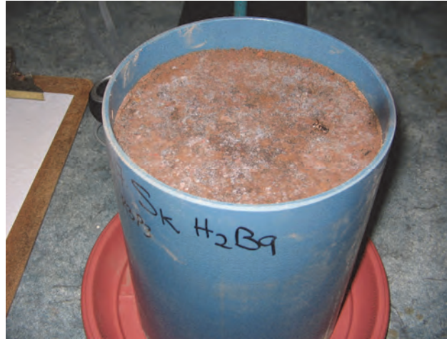
Figure 10.5. Salt-like precipitation on the surface of the fine sandy loam soil where winery wastewater augmented to 3000 mg/L were applied.
