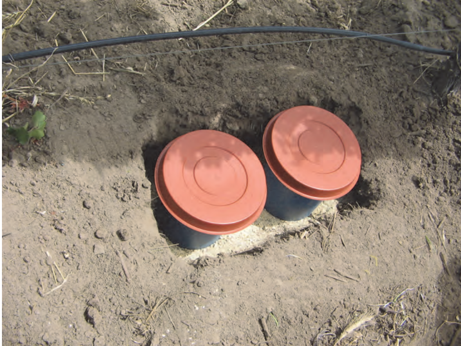
Figure 10.1. The PVC pots were covered with lids and placed onto a layer of coarse sand.
