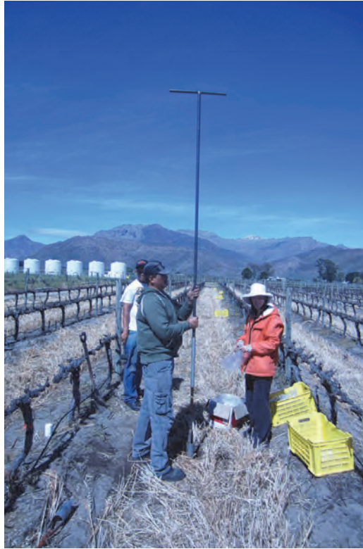
Figure 4.1. A modified soil auger, which was used to collect soil samples to 3 m depth.
