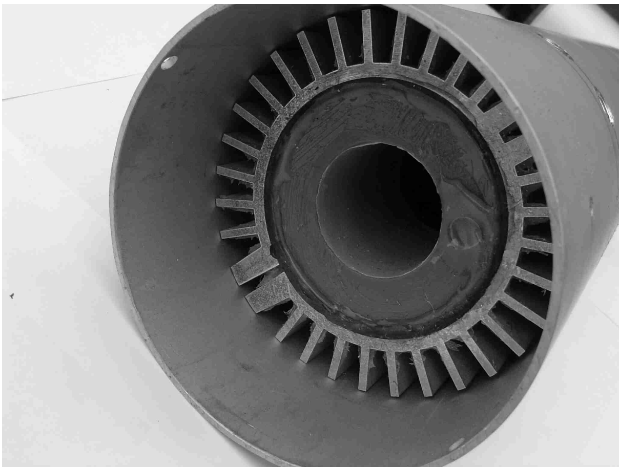
Figure 13: Air-cooled electrode structure
