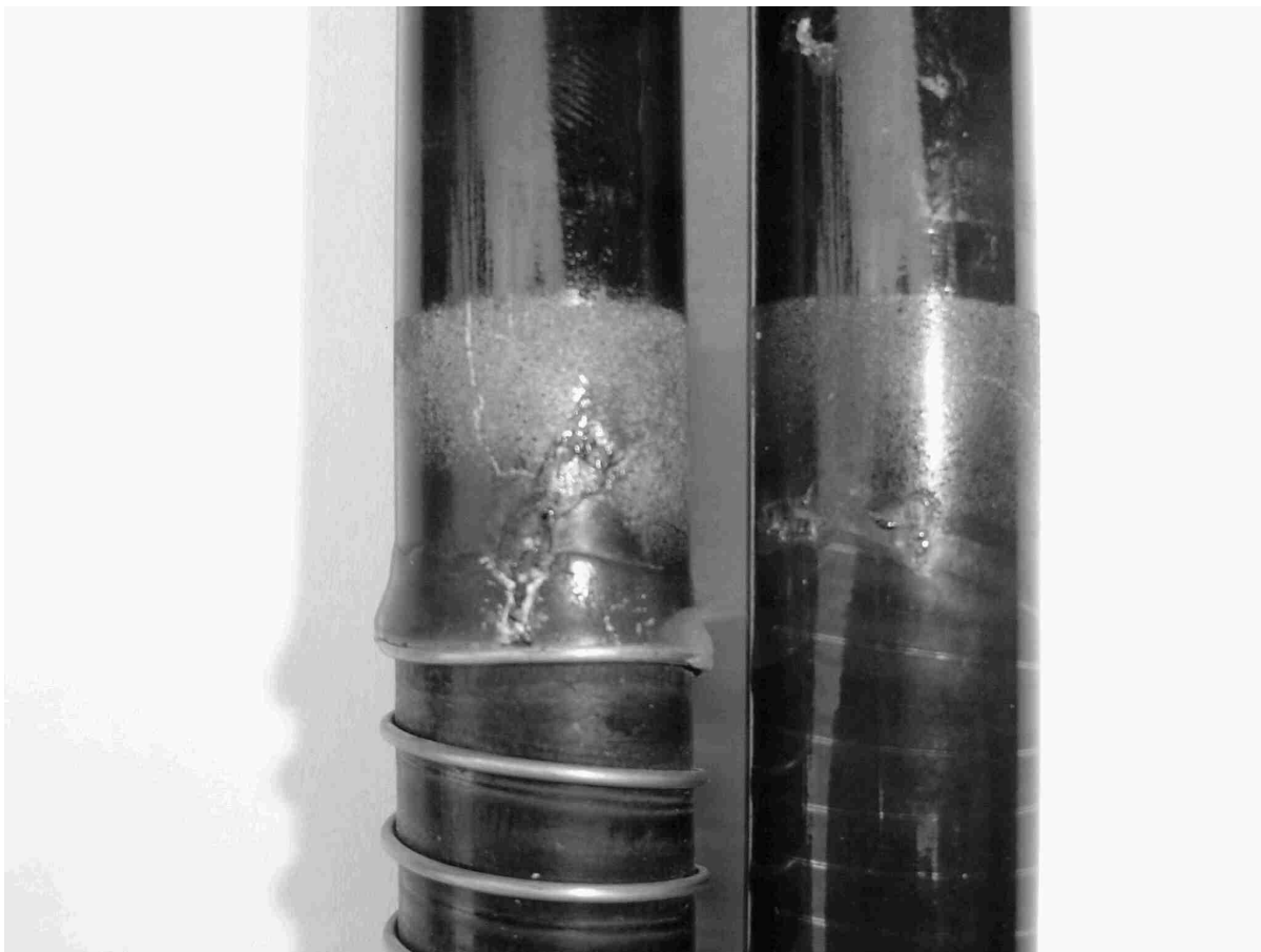
Figure 8: Examples of corrosion damage to electrodes
