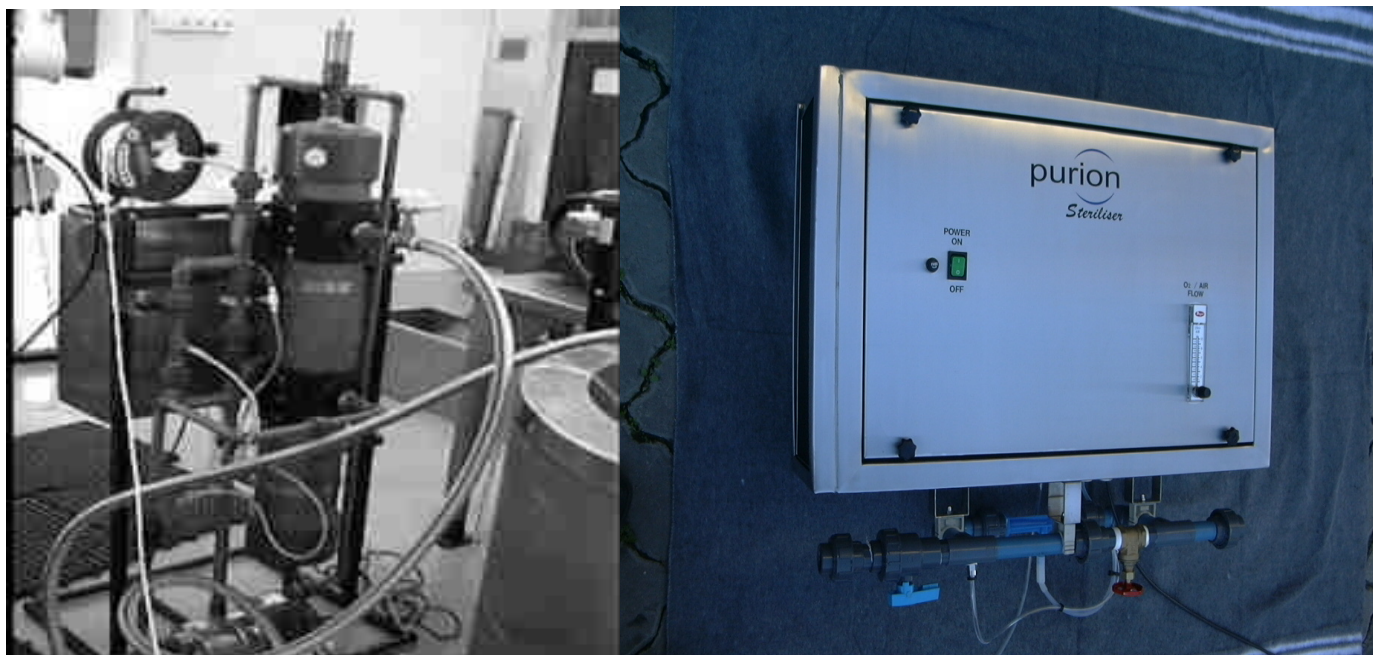
Figure 18: Two general-purpose ozonation systems using the PURION technology
