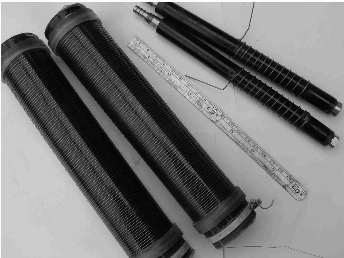
Figure 6: Ceramic layer applied to the metal ground tube, and a selection of complete electrodes
