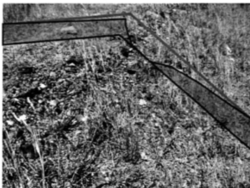
Figure 12: Slumping of the soil cover and erosion frequently result in exposure of underlying coal discard at the top of terrace slopes. Solid brown line indicated soil cover at placement. The fill represents the actual soil cover ten years after rehabilitation
