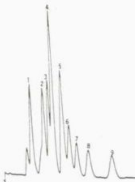
Figure 5.24: High pressure liquid chromatogram of volatile fatty acids standard solution containing 1: citric acid; 2: lactic acid; 3: formic acid; 4: acetic acid; 5: propionic acid; 6: iso-butyric acid; 7: n-butyric acid; 8: iso-valeric acid; 9: n-valeric acid
