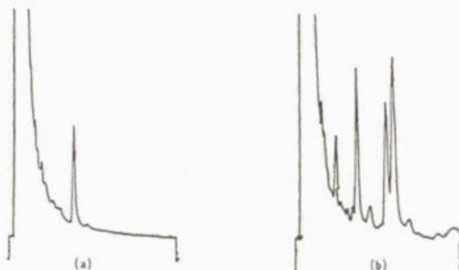
Figure 5.17 : Gas chromatographic separation of B-HO butyrate methyl ester (a) B-HO butyrate methyl ester; (b) mixed liquor containing B-HO butyrate methyl ester
