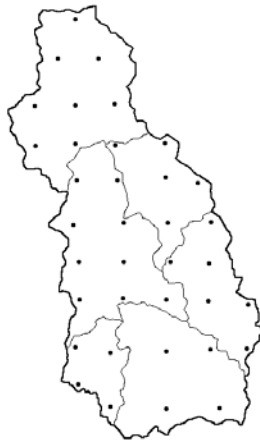
Figure 3.6: Approximate positioning of the Liebenbergsvlei rain-gauge network on the six Quaternary sub-catchments.
