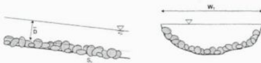
Figure 14: Definition sketch for Jonker's large-scale roughness equation. (Jonker, 2002)
