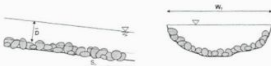
Definition sketch for Jonker's large-scale roughness equation. (Jonker, 2002)
