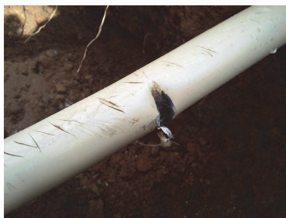
Plate 4.10: Gas line damaged by a new fence pole inserted into the ground at Obonjaneni, KZN.
