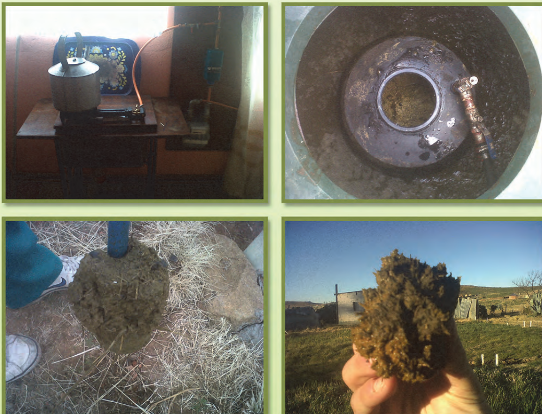
Plate 6.1: Clockwise from top left: (a) High gas pressure, minimal gas, (b) opened gas chamber, (c) solid mass of ligneous material, and (d) light fluffy consistency of the ligneous material
