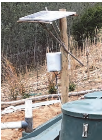
Plate 2.5: BiogasPro Meter installed at Okhombe pilot household, KZN.
