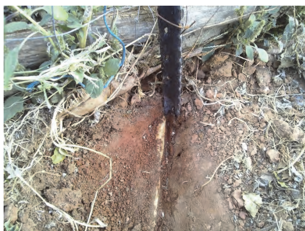
Plate 4.10: Gas line damaged by a new fence pole inserted into the ground at Obonjaneni, KZN.
