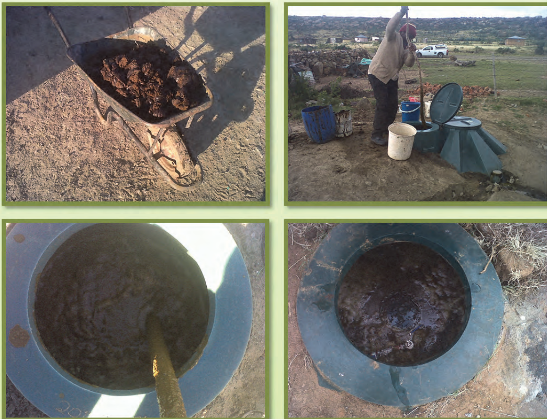
Plate 6.3: Clockwise from top left: (a) cattle dung serves as the primary feedstock, (b) additional mixing of feedstock within the biodigester, (c) consistency of the feedstock is very thick and additional water is added and (d) evidence of overloading the digester.
