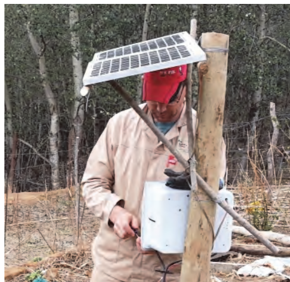
Plate 2.5: BiogasPro Meter installed at Okhombe pilot household, KZN.
