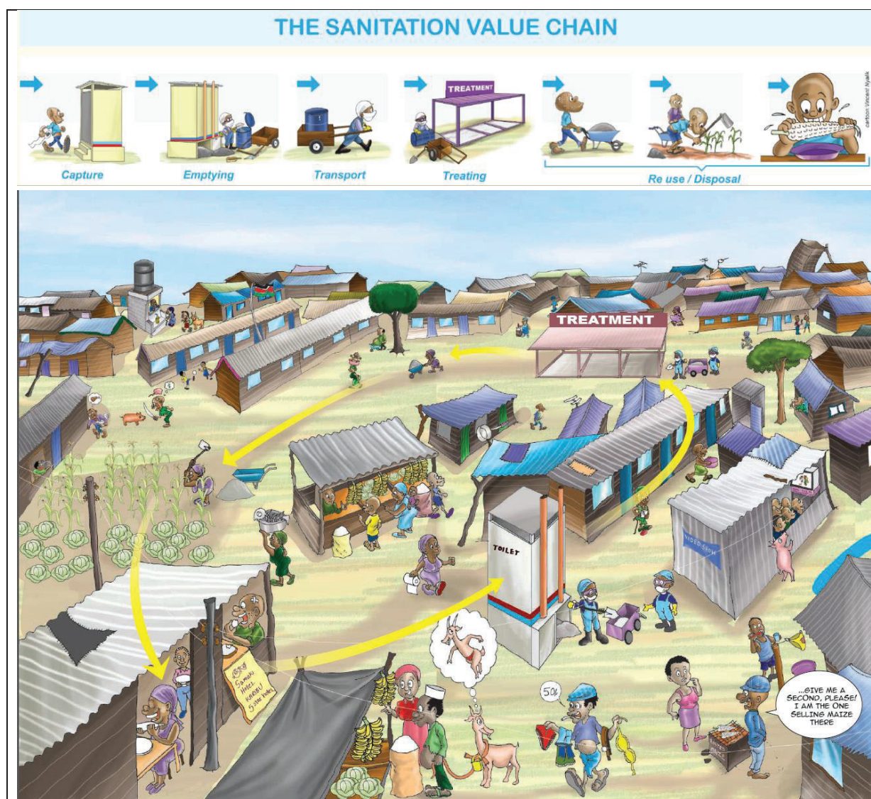
Figure 4-5: Sanitation value chain with manual treatment of sanitation waste (Image compiled from various SafiSan posters [Water Sector Trust Fund])
