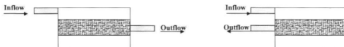
Diag. 4.1: Different ways of water flow through filters
