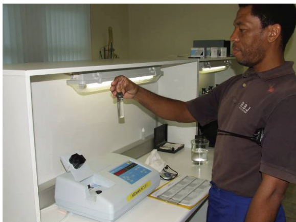
Operational monitoring equipment is required to track turbidity, pH and chlorine concentrations through the plant
