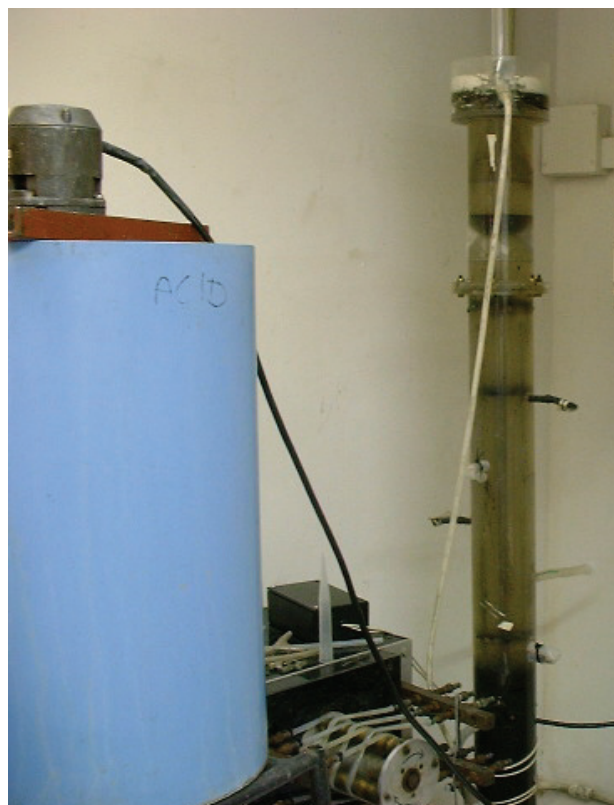
Figure 3.2: Laboratory-scale UASB system for biological sulphate reduction with primary sewage sludge as substrate.
