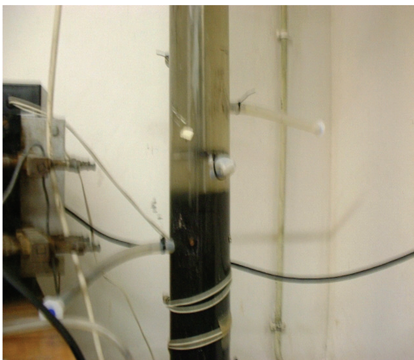
Figure 6: Sludge bed separation in the laboratory-scale UASB reactor.
