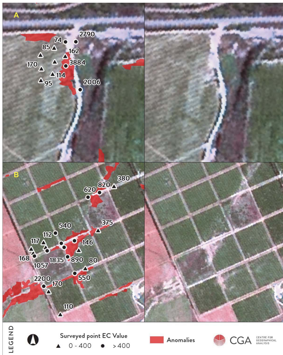
Figure 6.15 Examples of anomalies detected at Sundays River that were confirmed to be related to waterlogging and/or salt accumulation.
