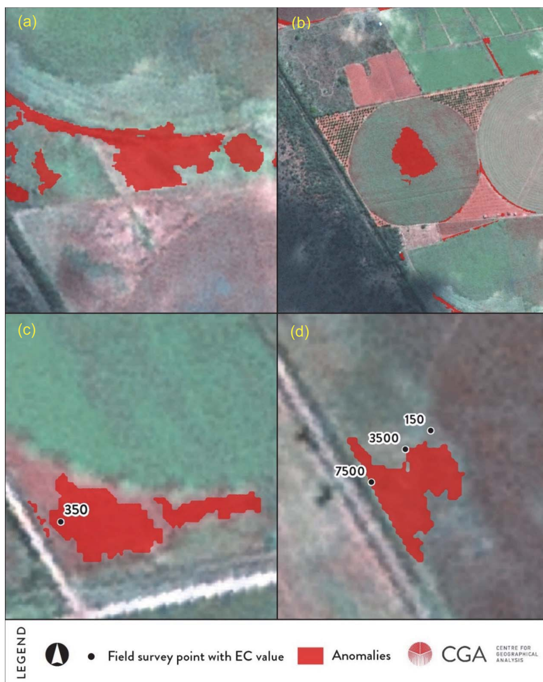
Figure 6.3 Examples of areas at Vaalharts where within-field anomalies were detected for the period 2010-2012.
