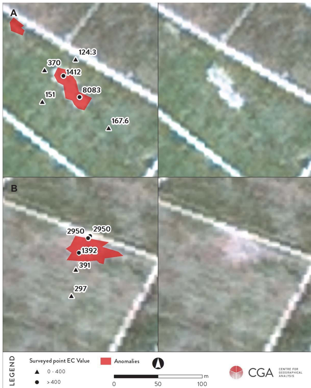
Figure 6.14 Examples of small anomalies detected at Breede River that were confirmed to be related to waterlogging and/or salt accumulation.
