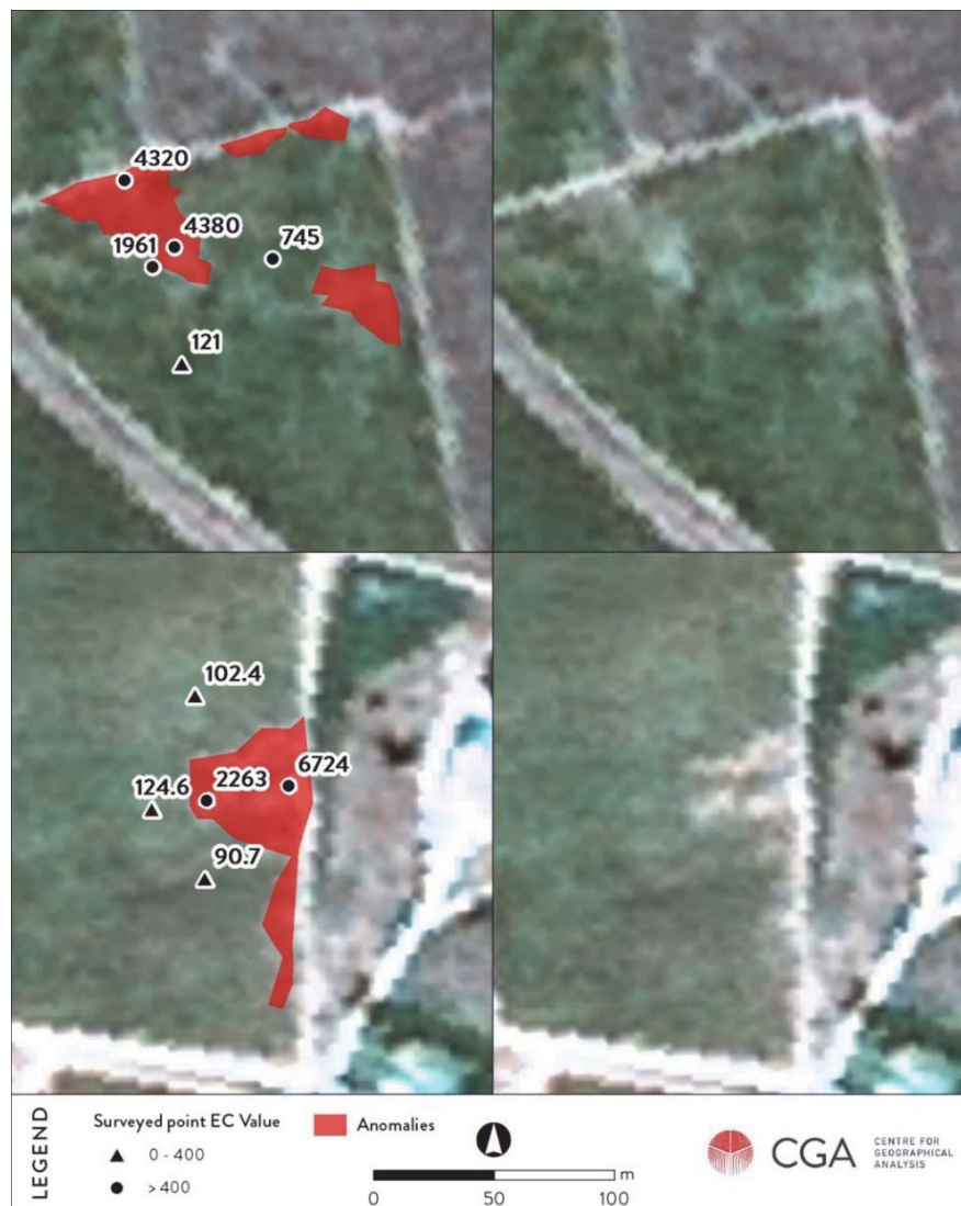
Figure 6.13 Examples of large anomalies detected at Breede River that were confirmed to be related to waterlogging and/or salt accumulation.
