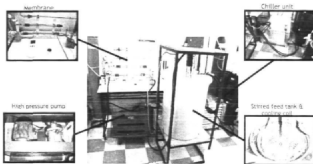
Figure 9: SPARRO Membrane Test Rig (SMTR) photograph
