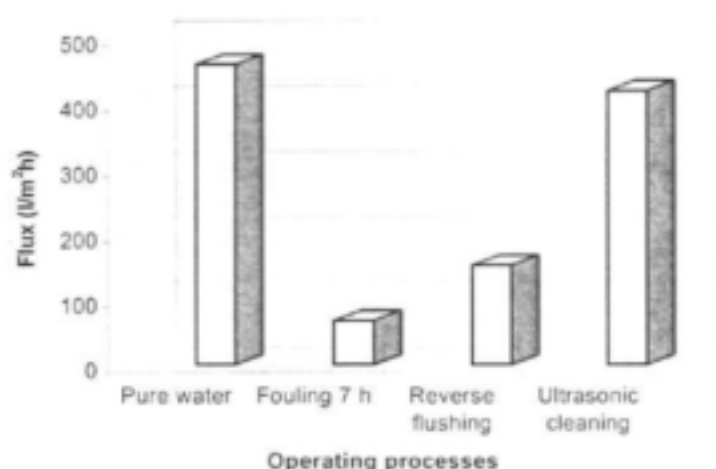
Figure 5.8: Change in flux during fouling and cleaning processes (at pressure 100 kPa and flow rate 6.07 cm/s).
