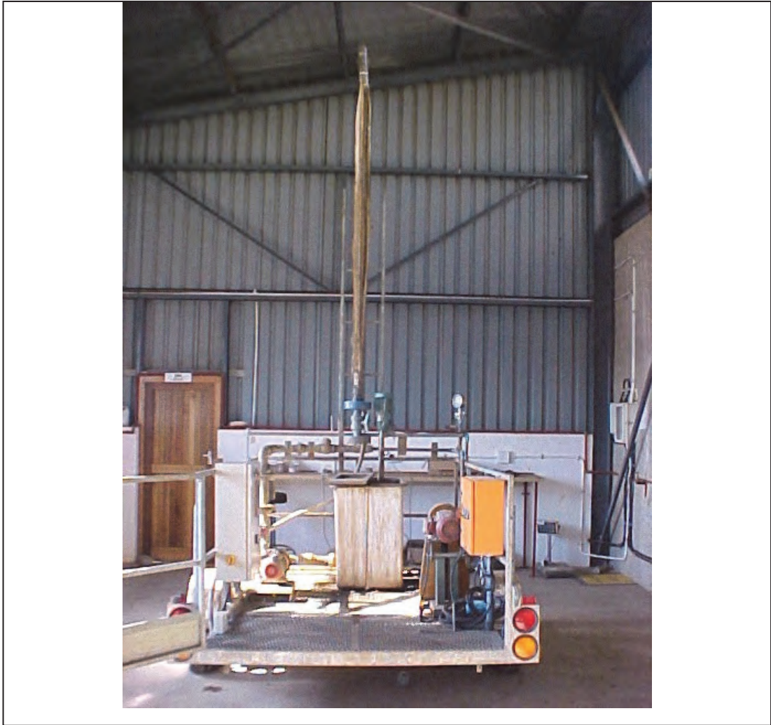
Figure 3.2: The Single Tube Pilot Plant
