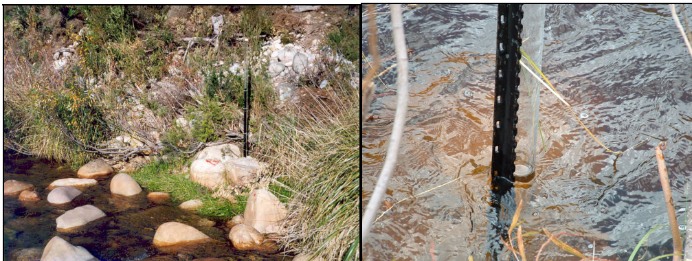
Figure 6: Plastic Stage Pipe used to Measure Flood Levels
