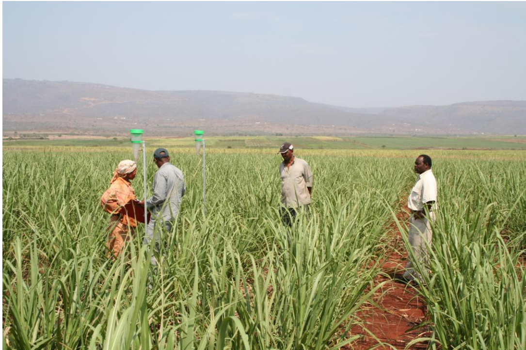
Figure 4.3 Makhathini participants are shown how to capture rainfall and irrigation data as well as wetting front detector responses.
