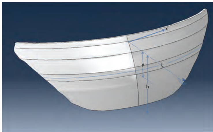
Figure 5.2: The parameters used to describe the added mass in the USBR Manual.
