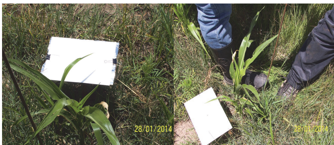
Figure 4.3: Chromatography paper (27 × 15 cm) mounted 20 cm above the ground and held in place with clamps on an aluminium surface for spray drift deposition sampling.
