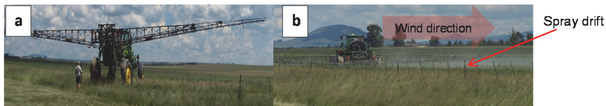
Figure 4.1: (a) The ground sprayer with 56 nozzles along a 32 m boom used to apply the atrazine mix in Standerton (b) Visible spray drift away from the target crop during application.
