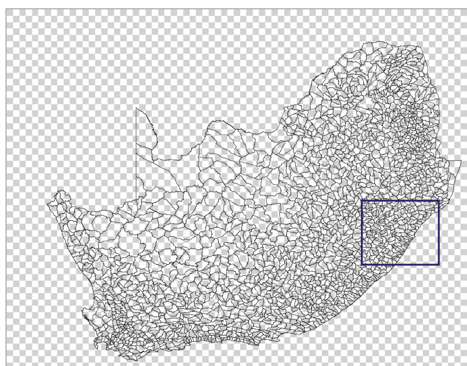
Figure 9.1 A 0.25° resolution grid overlaid by the Quaternary Catchment boundaries
