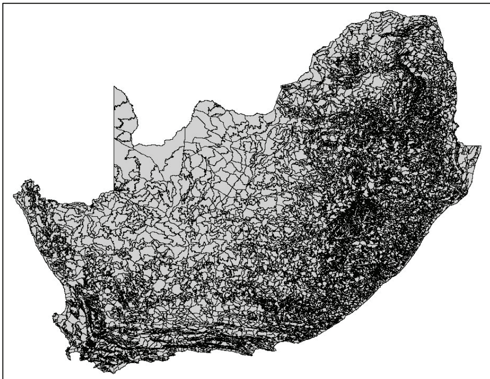
Figure 6.6 Delineation of the RSA, Lesotho and Swaziland into 5 838 hydrologically interlinked and cascading Quinary Catchments
