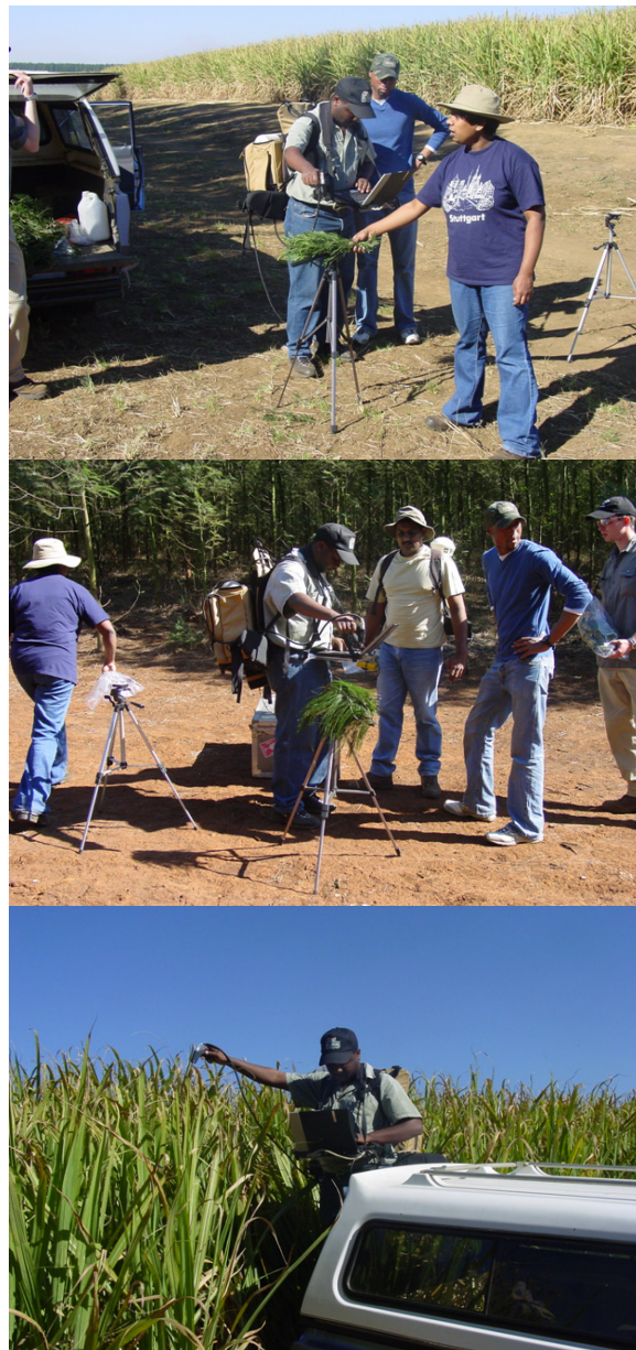
Figure 3 Hand-held ASD spectral reflectance measurements from wattle leaves, pine needles and sugarcane.
