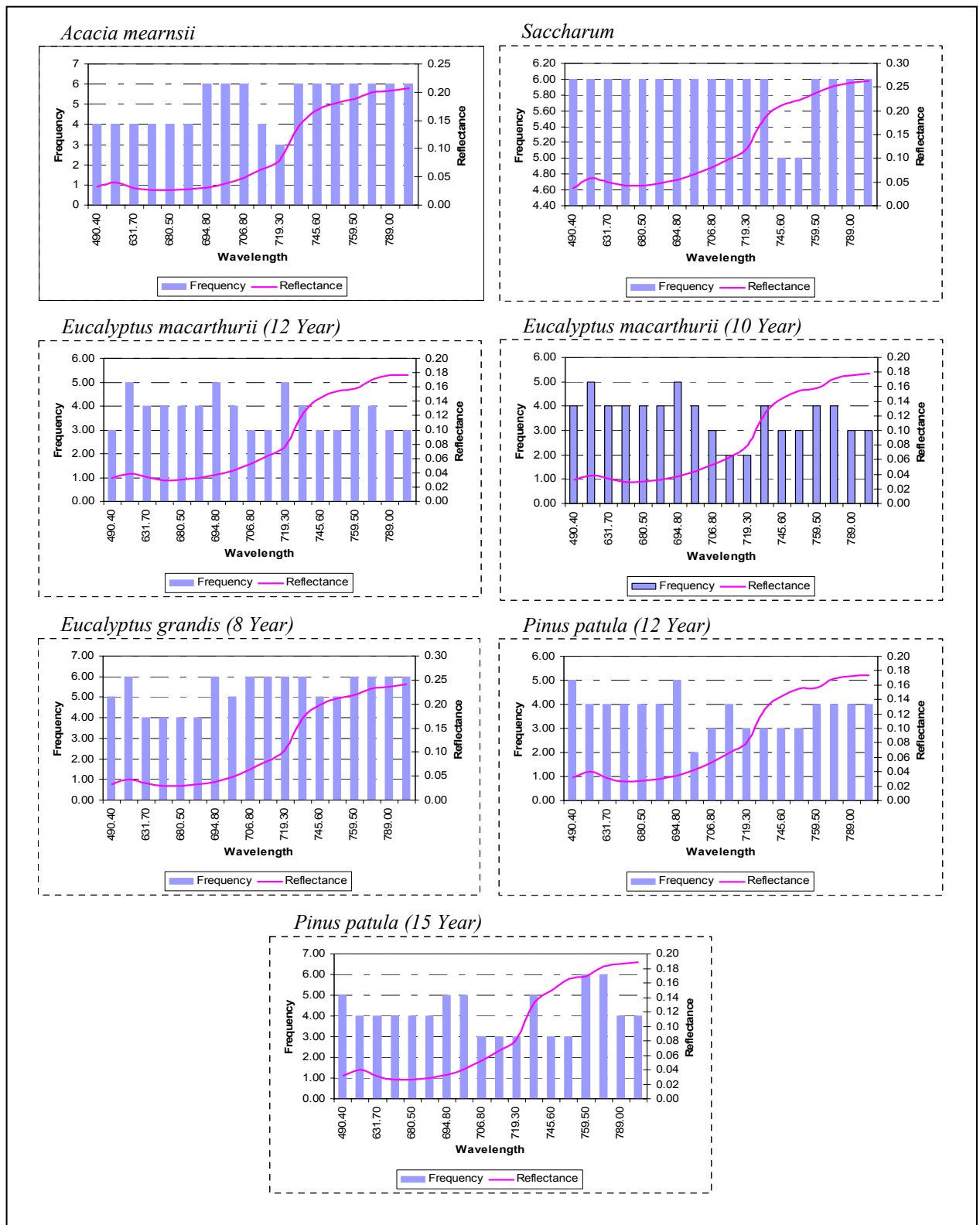
Figure 8 Frequency distribution of the significant spectral bands and the average spectral reflectance signature for individual classes extracted from Proba Chris image acquired in summer 2007.
