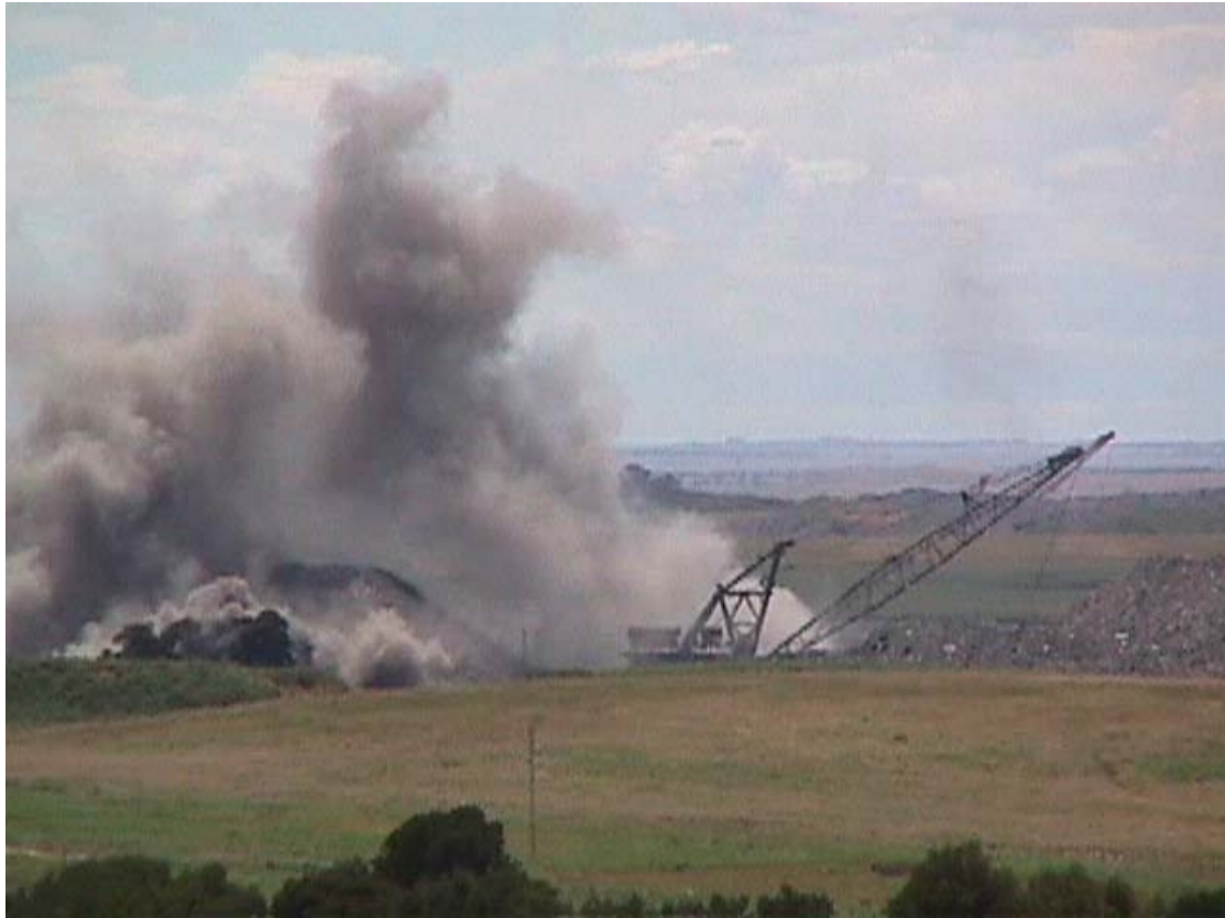
Figure 25. Dragline mining in an opencast pit .
