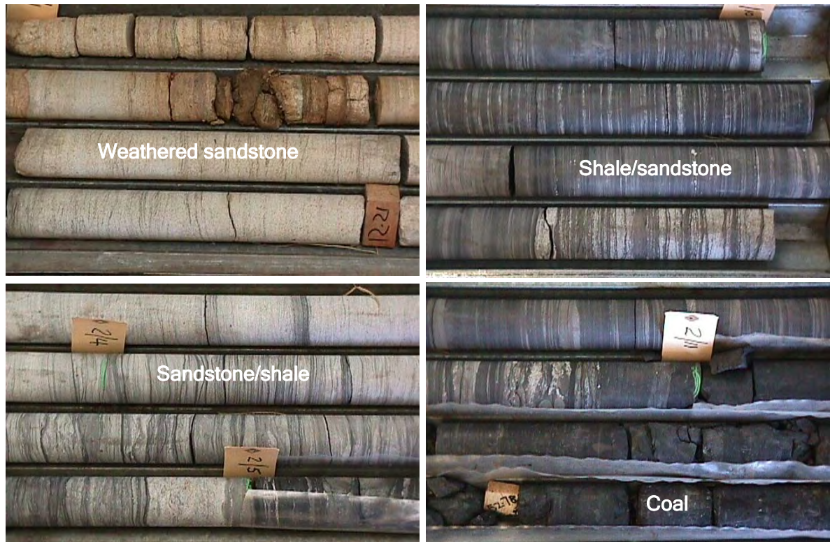
Figure 13. Photographs of typical sedimentary rocks from the Mpumalanga Coalfields.
