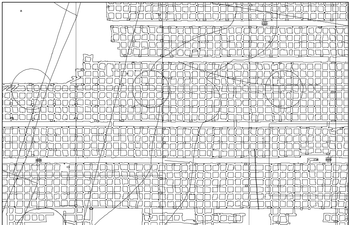
Figure 14. Example of bord-and-pillar mining in a modern underground colliery. Apart from the coal pillars, certain surface infrastructure such as streams, roads and survey markers are also shown.
