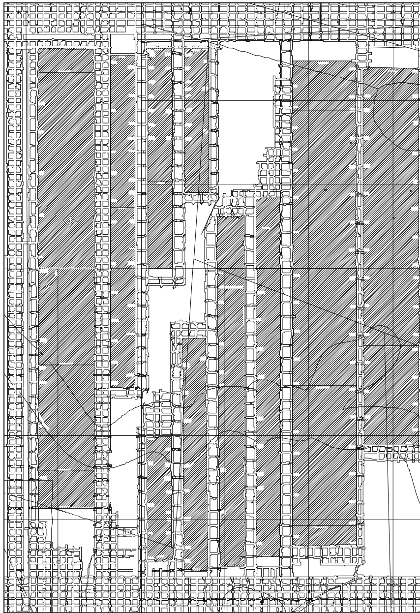
Figure 22. Example of longwall panel lay-out with a structural discontinuity transecting it, also showing bord-and-pillar mining to allow access.
