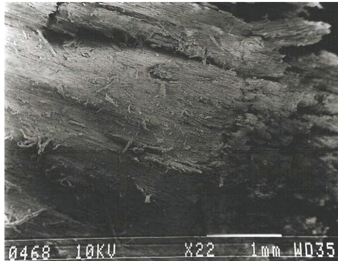
Figure 4.37: SEM of the woodchip sample from the Middle layer (22X).
