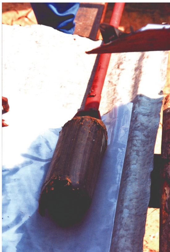
Figure C-11: Carbon auger containing extracted carbon.
