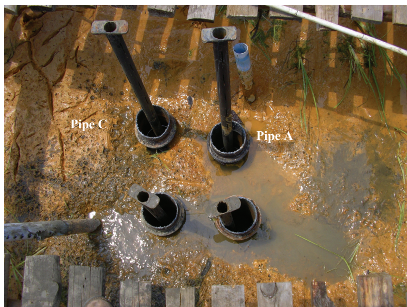
Figure C-9: Placement of the carbon sampling corers (only pipes A and C were successfully sampled).
