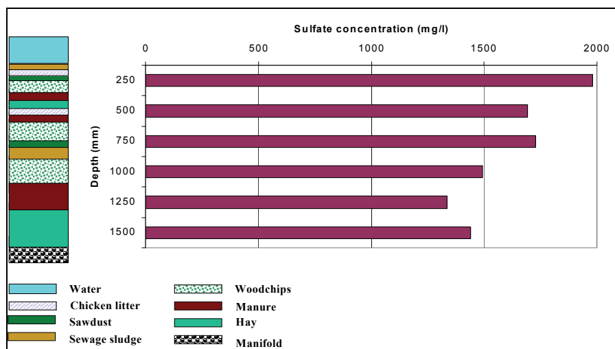
Figure 4.7: Sulfate concentrations over the depth of SSRU1.
