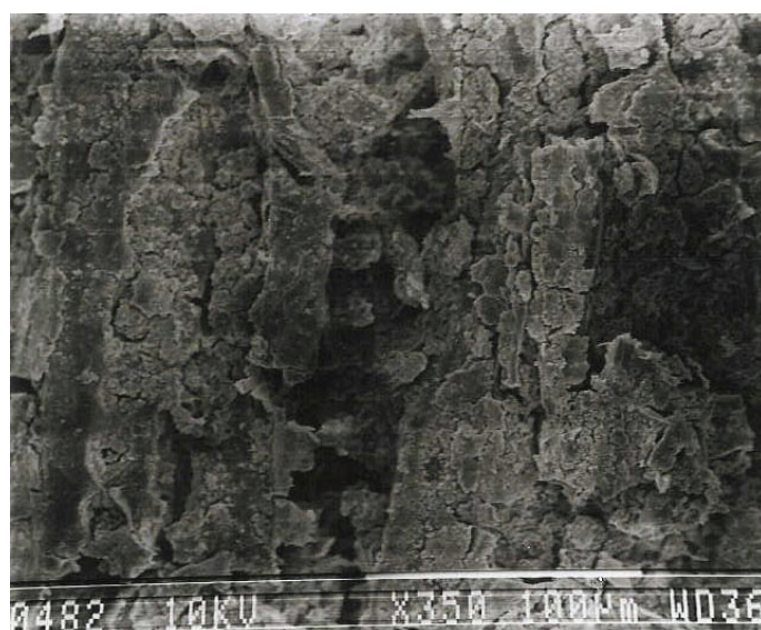
Figure 4.33: SEM of the fresh wood control (350X).
