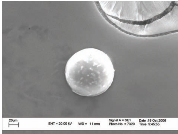
Figure 1: A PAN bead with a diameter of approximately 100 \mu\text{m}
