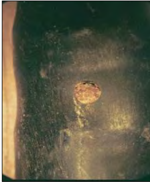
Figure 50: Soil in aperture
