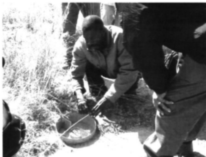
Plate 9. Splash cup used to measure up- and down- slope erosion.
