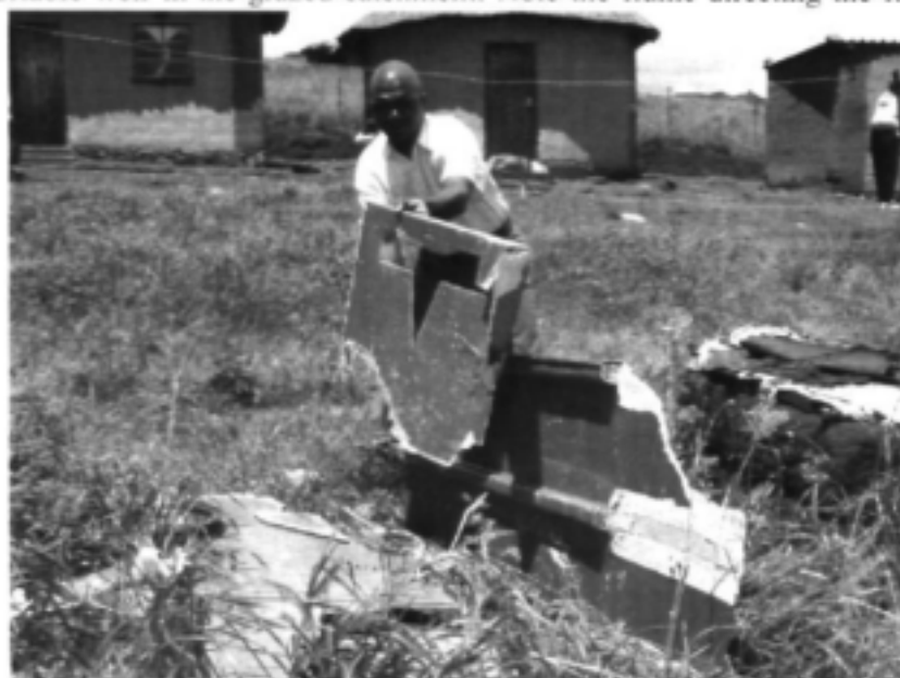
Plate 13. Portable weir in the grazed catchment. Note the flume directing the flow into the
