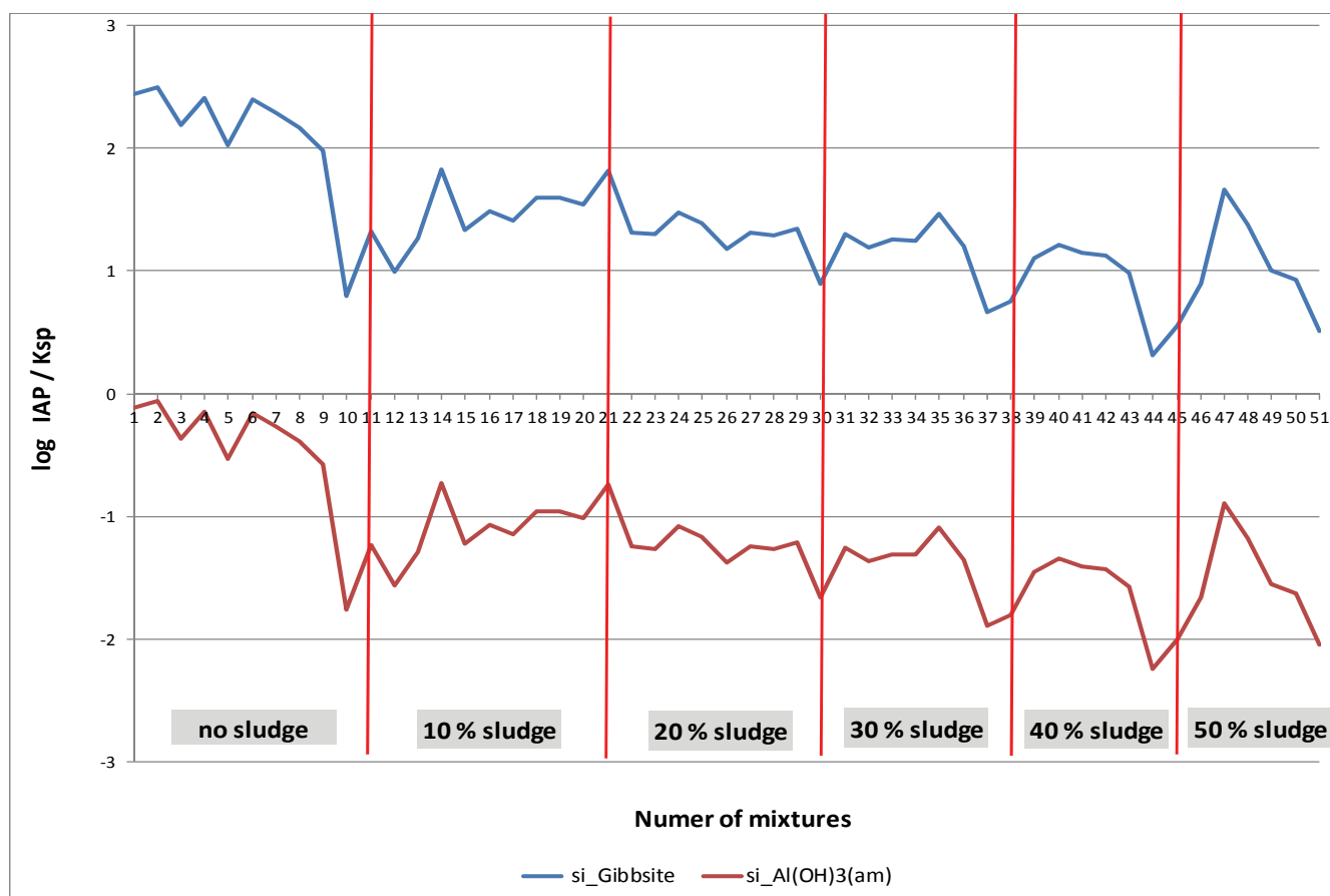
Figure 4.26 Gibbsite and amorphous Al(OH)_3 saturation indices of the various mixtures for the ninth leaching cycle. \log IAP / K_{sp} = 0 means solution is saturated with respect to a specific mineral, example, Gibbsite and this mineral can possibly control Al activity and availability
