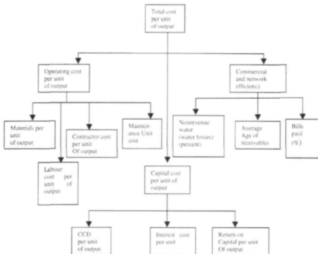
Figure 2 - Simple unit performance measures - Webb and Erhardt (1998)
