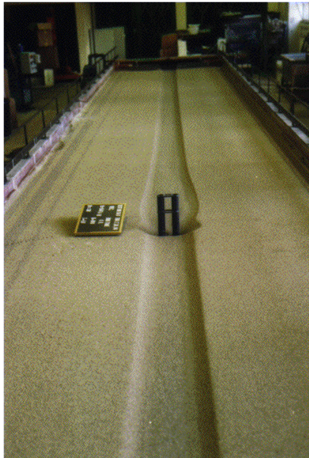
Figure 9-12: An example of equilibrium scour around a pier group (Babaeyan-Koopaei, 1996)
