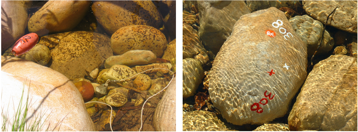
Figure 3.5 Example of a fish-marker marking the position of a stone and of a numbered stone repositioned on the stream bed.
