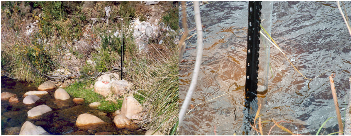
Figure 3.6 Plastic stage pipe used to measure flood levels.
