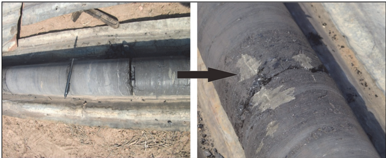
Figure 1-1: Core sample from exploration borehole near the GCM, with large pyrite hosted within the coal.
