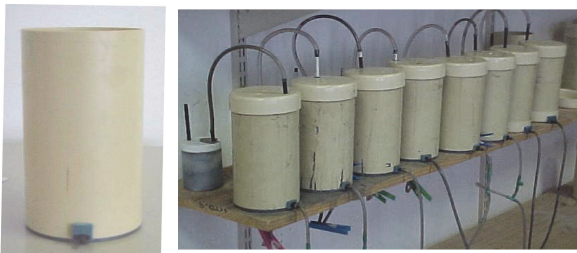
Figure 3-2: An IGS humidity cell, left and an array of cells set up at the IGS, right
