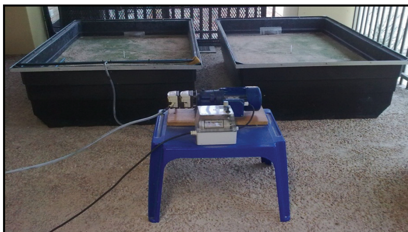
Figure B1 Photograph of two of the six sand-filled hybrid vertical-horizontal subsurface flow pilot-scale constructed wetlands at the Cape Peninsula University of Technology
