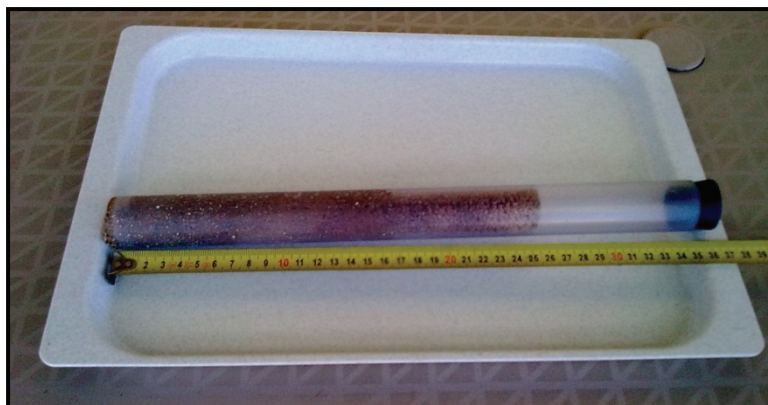
Figure B3 Photograph of core sediment sample, together with the Perspex corer and rubber bung used during the sampling procedure
