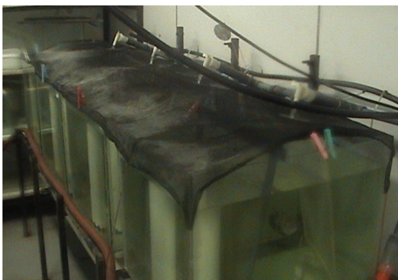
Figure 13B.1: Test organisms exposed to DDE concentrations in a continuous flow through system.
