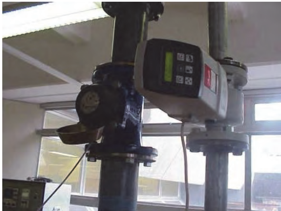
Picture 2: Water-meters used in laboratory: Mechanical for high flow-rates and magnetic for low flow-rates.
