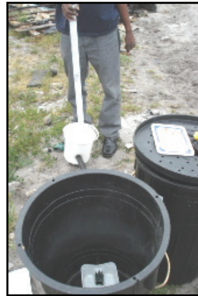
Figure 5.3: Preparation of a drum filter with a sampling bucket
