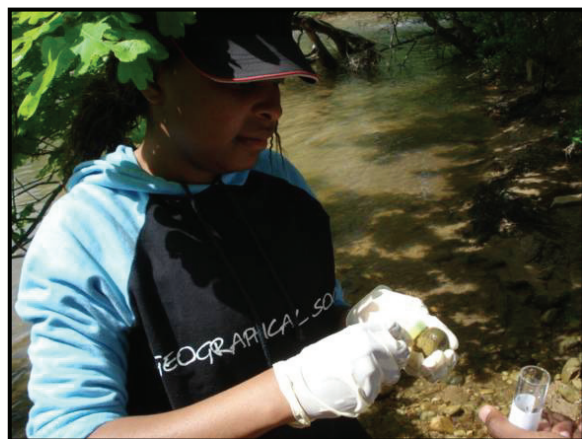
Figure A.3: Researchers collecting samples – diatoms from underneath a small rock at Site B (left); and water samples for chemical analysis at site A (right)
