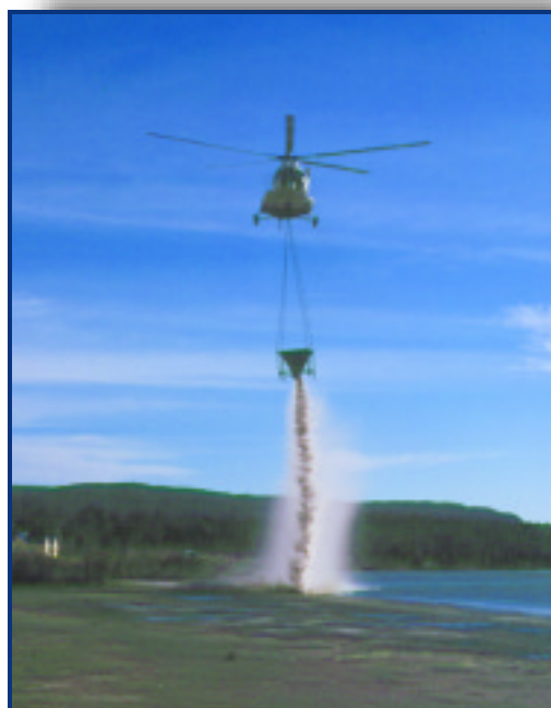
Wilde voëlvlei - by using helicopters to "bomb" the vlei with coarse rock salt, the salinity levels in the vlei were manipulated, eradicating the microcystis bloom.
