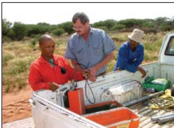
Johannes Haas (left), scheduling assistant, is one of two working out of Douglas. Here he sorts out a minor problem with a neutron probe cable under the watchful eye of Andries Wiid and a farm foreman. Absolute reliability is essential and requires discipline, organised training and support at all times.
