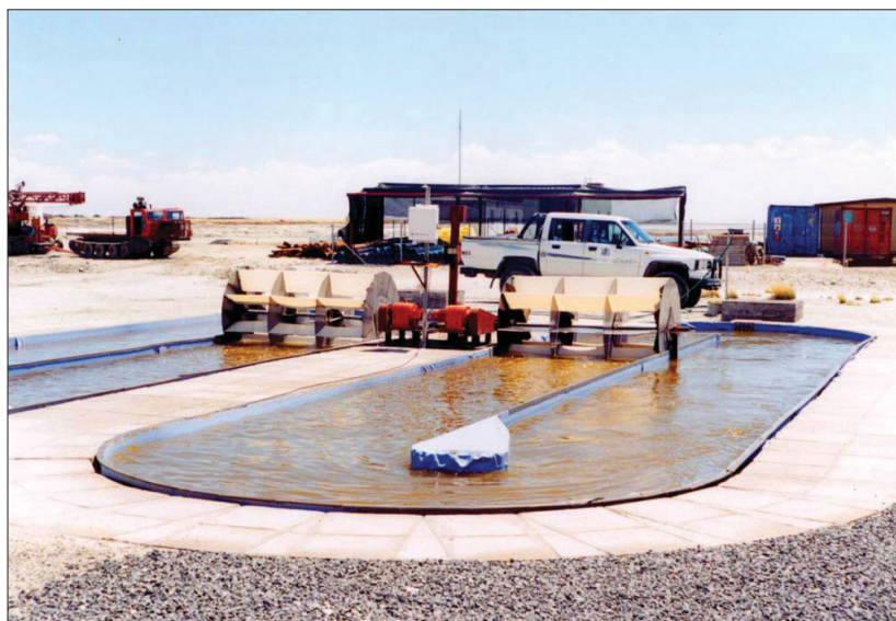
The Dunaliella high-rate algal pond pilot plant treating saline carbonate brines at Botswana Ash Co, Sua Pan.
