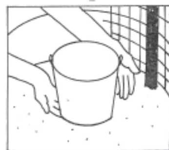
Place the bucket (bottom removed) on the ground in the middle of the tower.
